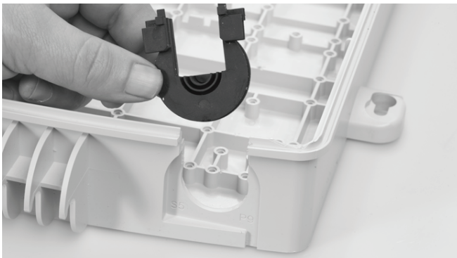
1.5 Use a hacksaw to reach the onion rings, which can be opened with a plier to open the in-line ports (S4/S5).
