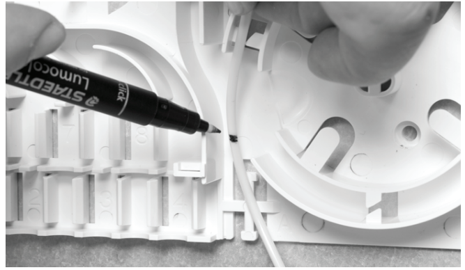
2.1 Mark the loose tube at the position of the tray.
