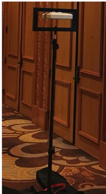
FIGURE 4: RUCKUS-DESIGNED SITE SURVEY STANDS ON TRIPODS
