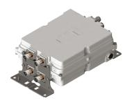
Dual Band Tower Mounted Amplifier, 1800//2100 MHz, 12 dB, 2 BTS & 4 ANT ports, with 4.3-10 connectors, AISG with 1 RET connectors (2 devices with 2 sub-units each)
