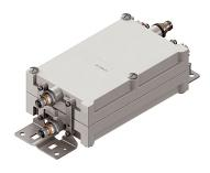
Dual Band Tower Mounted Amplifier, 1800/2100 MHz with 1400 MHz bypass, 12 dB, 2 BTS & 2 ANT ports, AISG with 1 RET connector (2 devices with 2 sub-units each), with 4.3-10 connectors
