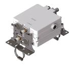
Dual Band Tower Mounted Amplifier, 2100//2600, 12 dB, 2 BTS & 2 ANT ports, AISG with 1 RET connector, with 4.3-10 connectors (1 device with 2 sub-units each)
