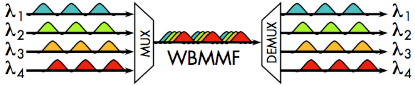
Figure 22. Shortwave division multiplexing over wideband MMF
